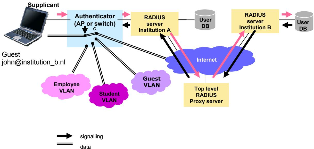
**Figure 1:** Authentication infrastructure for cross-domain authentication using 802.1X
